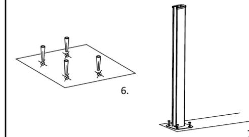
7. Make the left bottom hole of stand fix and the hole on the floor alignment and tighten them with M8x75mm hexagon wooden screw.
