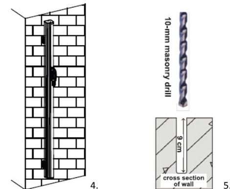
5. Drill four 10mm diameter holes on the floor in the size as shown in picture 5.
