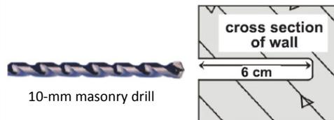
2. Insert one  $\varnothing 10 \times 50$ mm anchor bolt in each of the holes.
