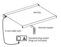
Once the power goes to the motor, give it 5 seconds, then press "P2", twice then press "OPEN" (on the back of the remote zapper, remove cover), it will then be synchronised. If you want to change the direction, turn the power off, and after 10 seconds, turn the power back on. 5 seconds later press "P2" twice and "CLOSE" (on the remote zapper), you will find the directions have changed.
