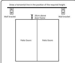
If in doubt about the quality of the wall structure you are wanting to mount the awning on, you can use an epoxy resin product to secure the mountings in the wall.
